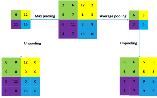
Figure 8. Example of Unpooling
